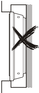
Air circulation is blocked
